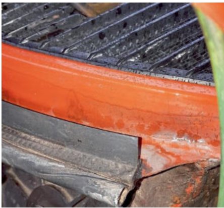
On opening the hood, it becomes clear that the paintwork on this Mercedes-Benz W 123 is not original
